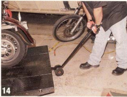
14 If the lift needs to be moved around, it comes with this cool wheel-dolly that has a fitting that connects to the back of the lift. This allows the lift to roll around without having to lift it, making it easy to move out of the way if needed.
